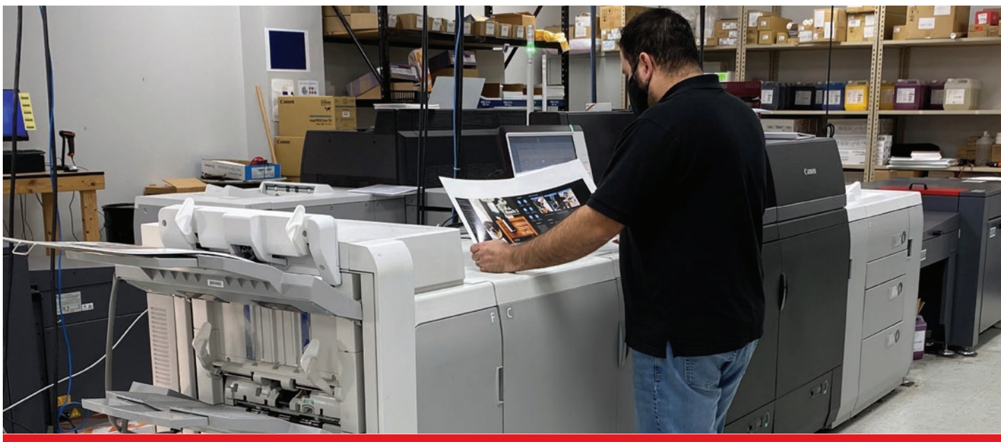
The Canon imagePRESS C10000VP cutsheet color toner press is equipped with a long sheet feeder to print up to 13" x 30" paper.
