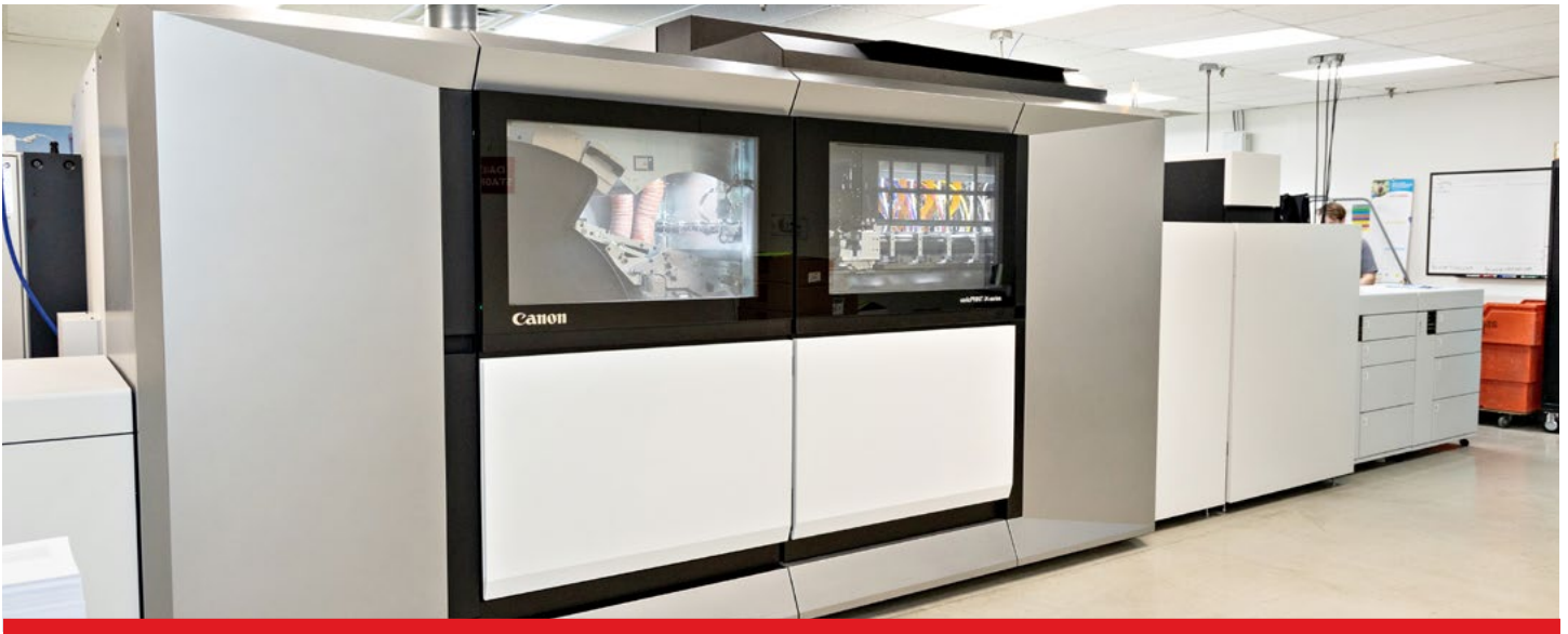
Two varioPRINT iX inkjet presses help Square One run 700,000 to 800,000 postcards a week with less labor and manual intervention, plus provide additional capacity for more work and larger jobs in a highly demanding environment.
