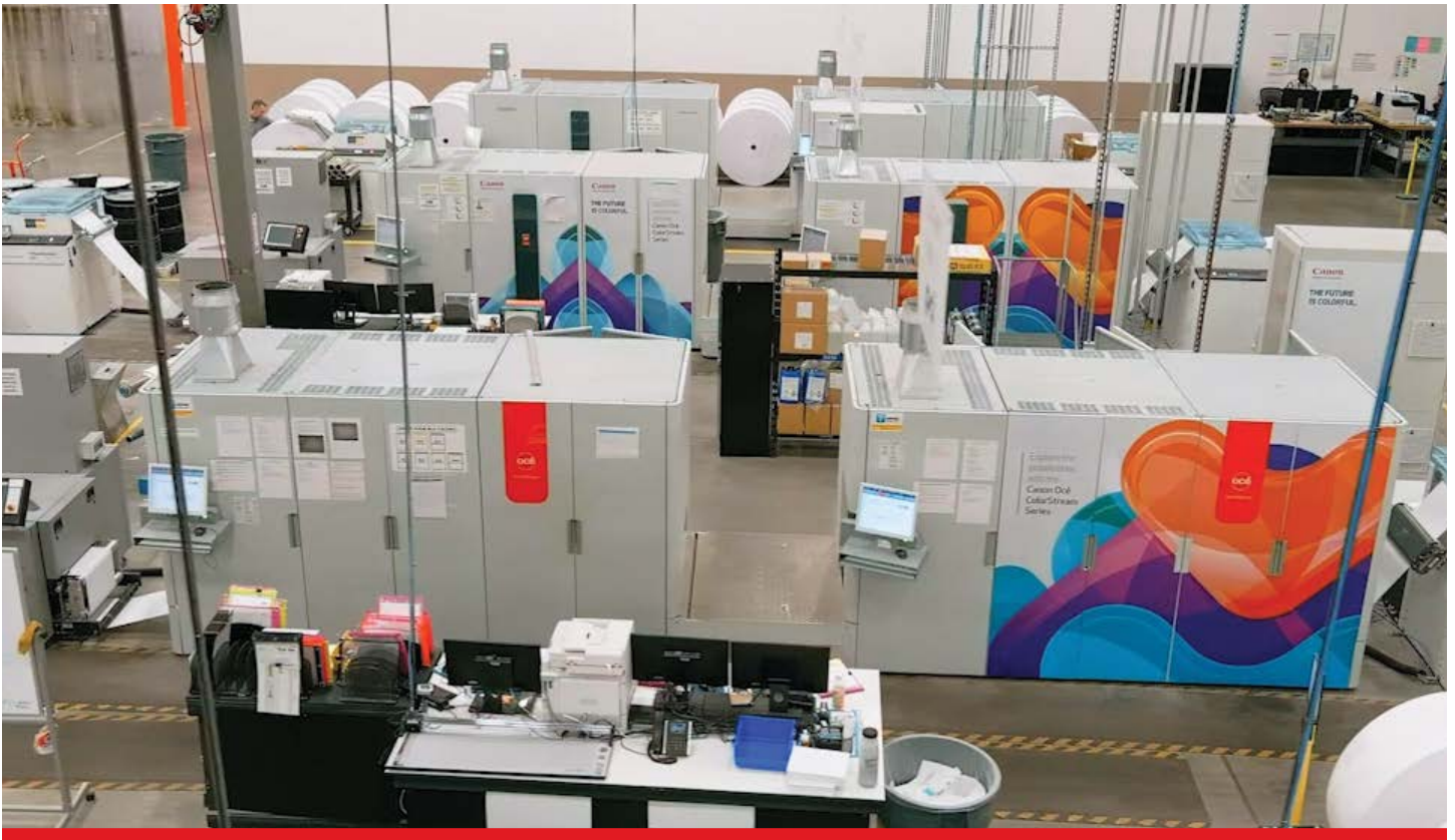
The PCI Group facility in Dallas features three Canon ColorStream inkjet web presses.
